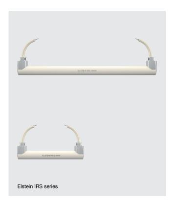
Elstein IRS rod radiators are ceramic infrared radiators, designed for operating temperatures of up to 650 °C. By the use of MPO/1 and MPO/2 mounting profiles, surface ratings of up to 72.0 kW/m² can be realised.
