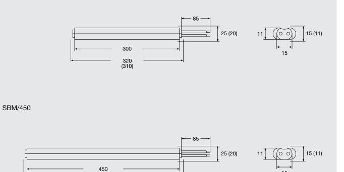
Mounting dimensions and radiator dimensions () in mm
