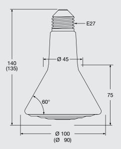
Mounting dimensions and radiator dimensions () in mm
